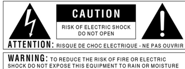
The above symbols warn the users of potential danger in case of misuse of electrical appliances. The thunderbolt in a triangle symbol shows that there is danger of electrocution. The exclamation point symbol shows that there are usage and safety measures which must be observed.
