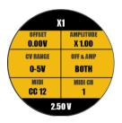
For **each CV output**, a **dedicated button** and **screen** allow you to quickly configure the output, **0.. 5V**, **0.. 8V**, **+-5V** as well as an **offset** and an **amplitude** coefficient. The voltage available on the jack is displayed in real time. You can thus adapt each CV information to the connected module.
