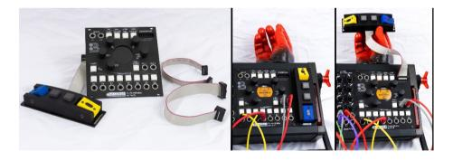
An optional self-powered external box is available to make the unit completely autonomous. It adds MIDI DIN out, USB MIDI In/Out, and a microSD card port .
